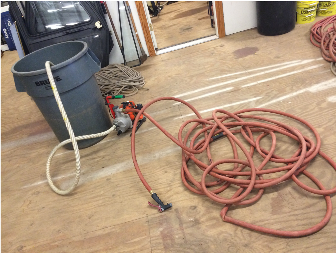
Figure 2. Spray rig used for SuffOil-X + Molt-X tank mix. Large garbage page was used for holding the mixed insecticide solution. Pump and hose were used for the delivery system.
